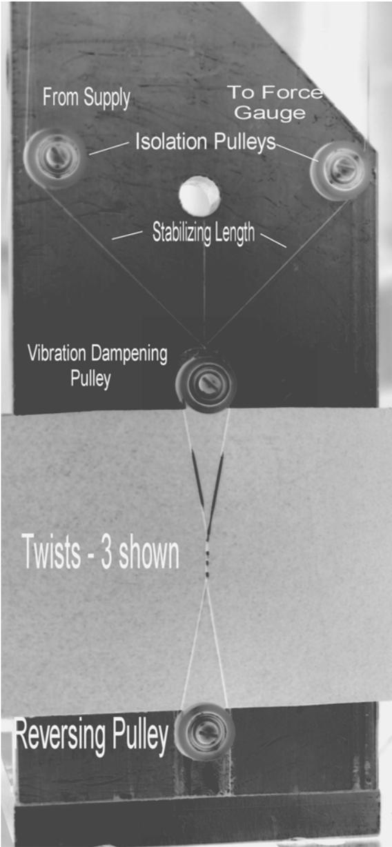
**Figure 3** Image of COF device with Fiber installed.
